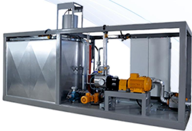
Asphalt Emulsions are bituminous binders formed by the dispersion of bitumen particles in water with the help of an emulsifier. Surface coating, bonding layer, primer etc. Asphalt emulsions, which have a wide application area, do not have flash points, they are not flammable and explosive.
